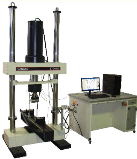
STD-600 with 3 Points Bending Fixture
