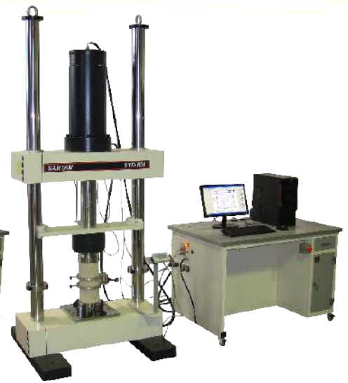
STD-600 with Compression Platens Self Align
